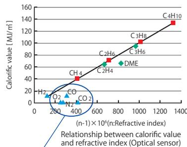
"Opt-Sonic calculation" using measuring results of the Optical sensor and Sonic sensor can minimize the interference effects caused by interference gases, and realize a high-accuracy measurement.
